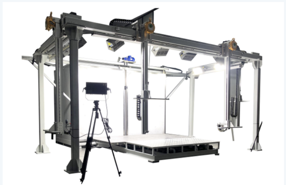
Auto Light & Camera Positioning System for Static Air Bag Deployment
